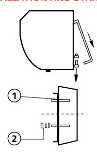
Unscrew the mounting plate and remove it.
