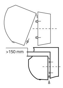
Position the mounting plate and secure it.
