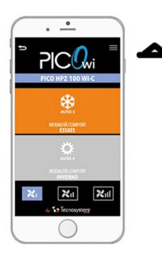
The system, set in Winter Comfort or Summer Comfort mode, is enabled, exploiting the temperature difference between the outdoor and indoor environment, in order to reach an ideal temperature in the indoor environment. You can choose between 3 available speeds.
