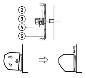
Unscrew the mounting plate and remove it.
