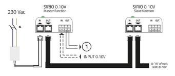
[1] Close with damper open, open with damper closed
