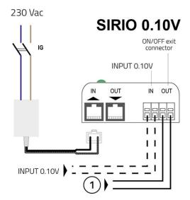
[1] Close with damper open, open with damper closed
