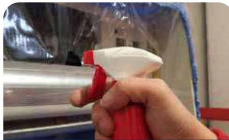
Battery cleaning through spraygun hole
