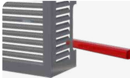
Preparation for passage conduit pipe and wiring
