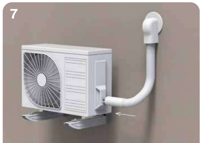
7 Flare the refrigerant pipes and fix them to the taps of the outdoor unit, connect the power supply. Approach and position the rubber sleeve near the taps.
