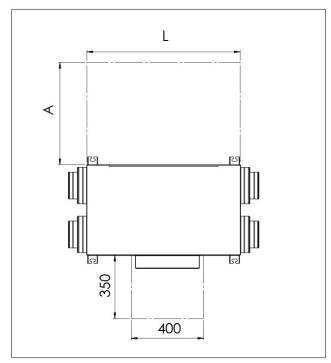
To make routine maintenance easier, provide a minimum access area as per the following table
