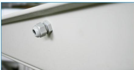
INSERIRE IL PASSACAVO NEL FORO POSTERIORE DELLA BACINELLA. / INSERT THE GLAND-NUT INTO THE REAR HOLE OF THE DRAIN PAN.
