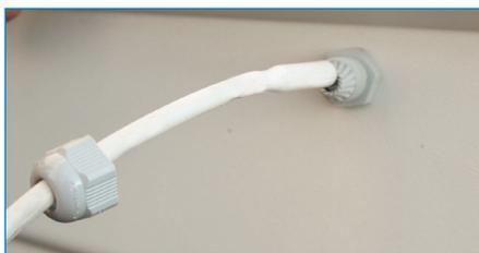
INSERIRE IL CAVO SCALDANTE NEL PASSACAVO. / INSERT THE HEATING CABLE INTO THE GLAND-NUT AND LET IT SLIDE TILL THE THERMOSTAT AND FASTEN IT.
