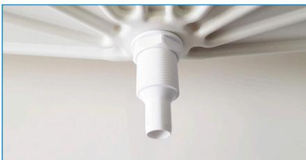
FISSARE LA PILETTA CON LA GHIERA FILETTATA INSERENDO LA GUARNIZIONE DI TENUTA ALLA BACINELLA. (CON CAVO SCALDANTE DA 6 m FAR PASSARE IL CAVO ALL'INTERNO DELLA PILETTA). / FIX THE DRAIN USING THE RING NUT BY INSERTING THE GASKET INTO THE DRAIN PAN. (WITH 6 M HEATING CABLE INTO THE DRAIN.)
