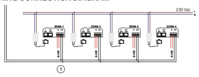
[1] 0-10V: controlled by home automation system or regulator 0-10V - the damper opens by modulating according to the voltage
