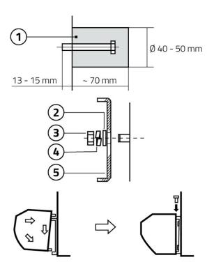
Drill a hole as shown in the instructions and insert the bolt into it, securing it with cement.
