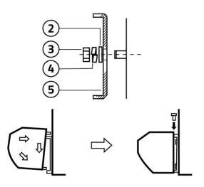
Drill a hole as shown in the instructions and insert the bolt into it, securing it with cement.
